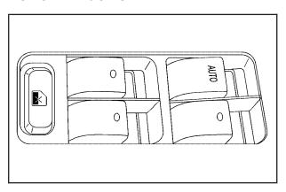
The switches on the driver's door armrest are used to control each of the windows. The power window switches work while the ignition is in RUN, ACCESSORY, or while Retained Accessory Power (RAP) is active. See *Retained Accessory Power (RAP) on page 113*. Each passenger door has its own window switch.
